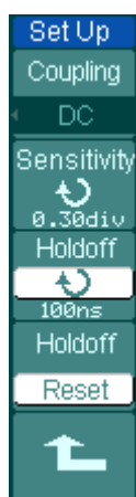
Figure 2-53 Table 2-32 The Trigger Set Up menu (Settings for trigger coupling, trigger sensitivity and Holdoff)
