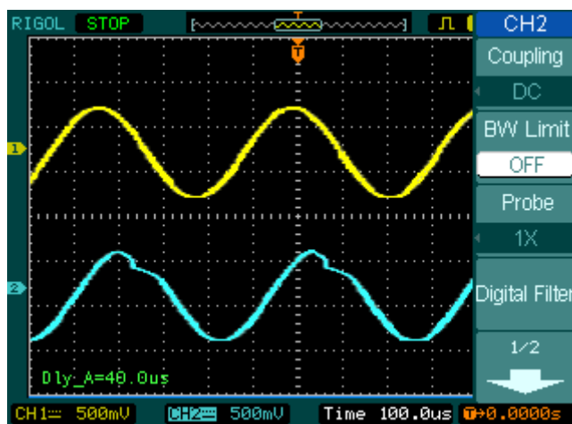
Figure 3-1 Delay of the signals
